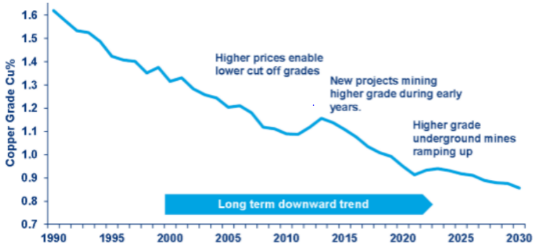
Copper Ore Grade Decline
