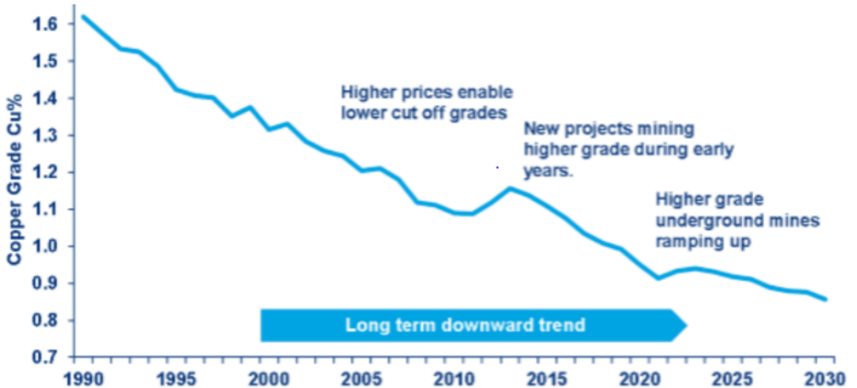
Copper Ore Grade Decline
